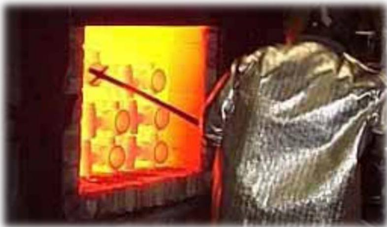
Burn-off & Shell Sintering in furnace
