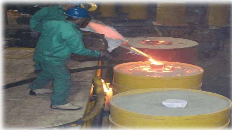
Metal Pouring in flask compacted with sand
