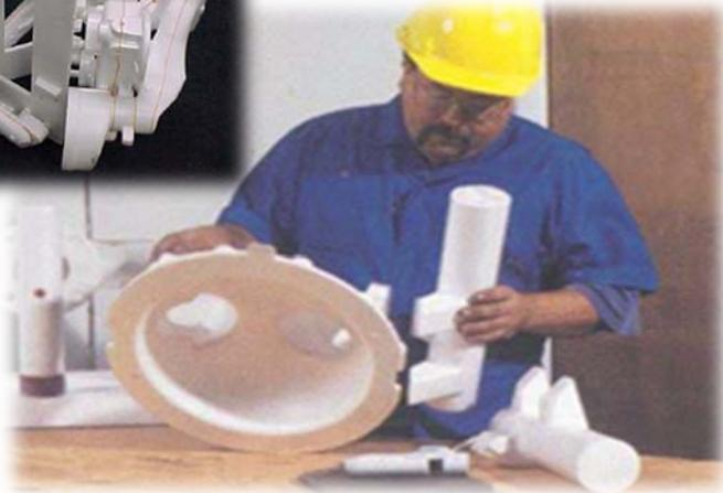
Gluing of Runners & Risers to foam patterns
