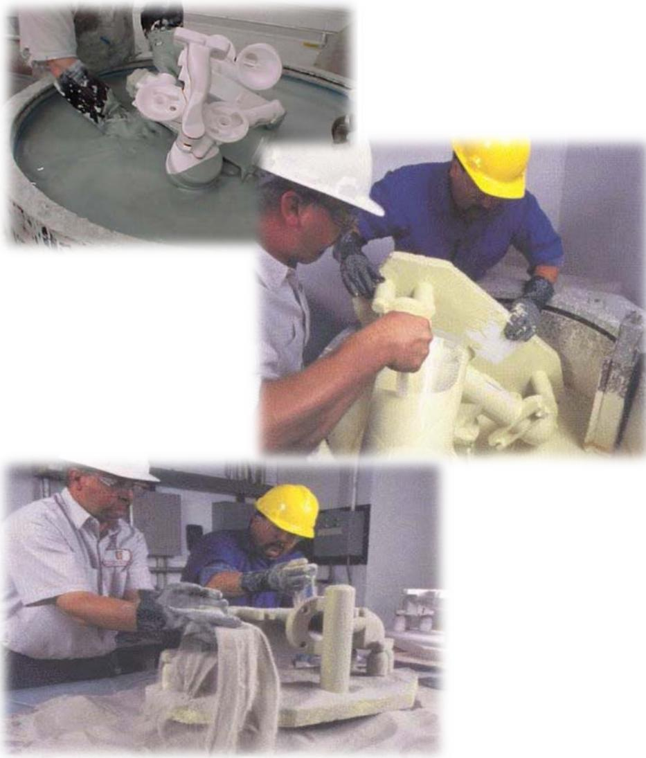
Coating parameters are verified before coating the patterns.
