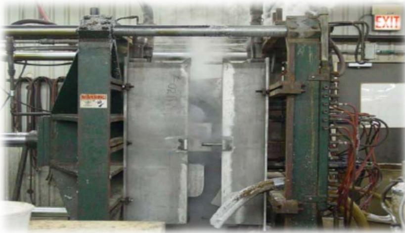
Foam Pattern Moulding on horizontal moulding machine
