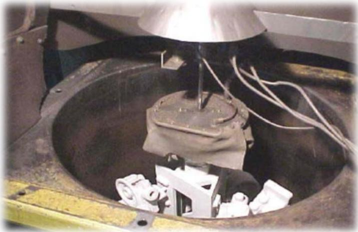
Shell placed in flask before pouring
